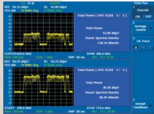
Simultaneous measurement of input/output for feed-forward amp
