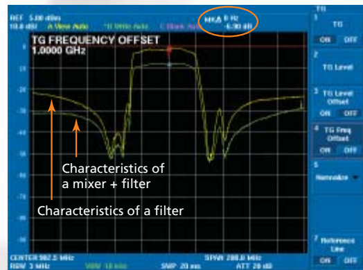
Measurement of mixer frequency conversion loss characteristics
